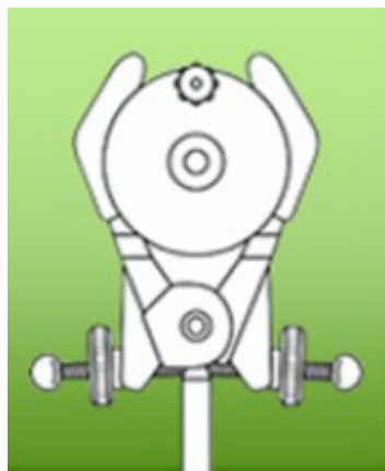
Figure 3 – Proper orientation of Envirochek capsule during the first cycle of the elution procedure
