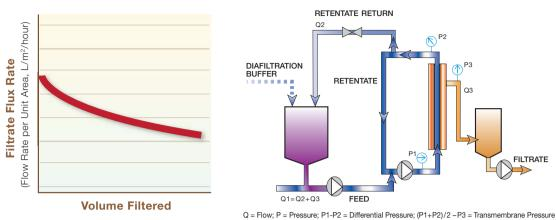
Examples of crossflow filters typically used in the food and beverage industry are the widely available systems using longitudinal modules consisting of polymeric (*e.g.* hollow fibers, spiral wounds) or inorganic (*e.g.* ceramic, sintered metal) membrane materials (Figures 8a–8b).
