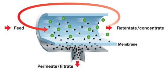
Figure 7a: Crossflow Filtration Principle: Feed flow direction is parallel to filtration surface and perpendicular to permeate flow direction.
