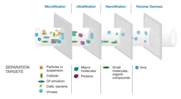
Figure 9: Filtration Spectrum of Crossflow Filtration and Separation
