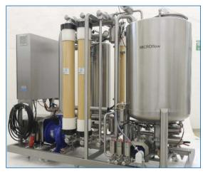
Figure 10d: Membralox Fermenter Broth Clarification System
